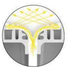
**(A)** Anidolic optical structures disperse and mix light, eliminating any visible images of the LED point source and ensuring accurate and consistent color.
